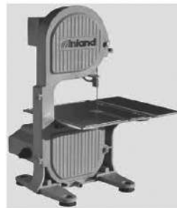
A continuous-band saw
